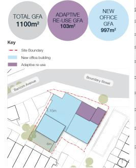
Figure 32. Option 2 Site Plan
